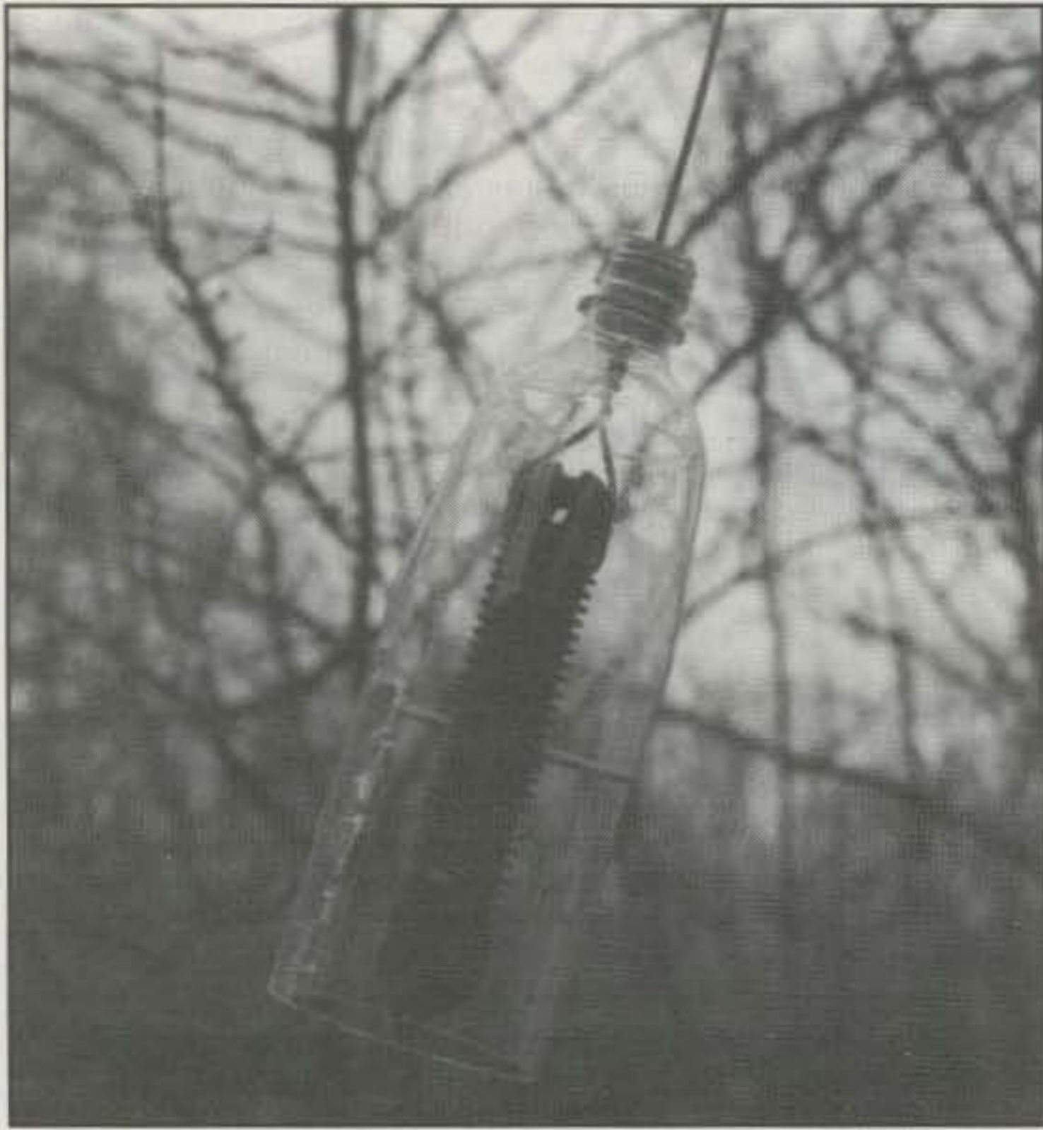
← Photo 6— "Bootie" protected end insulator used at bottom end of sloper or suspended vertical.
